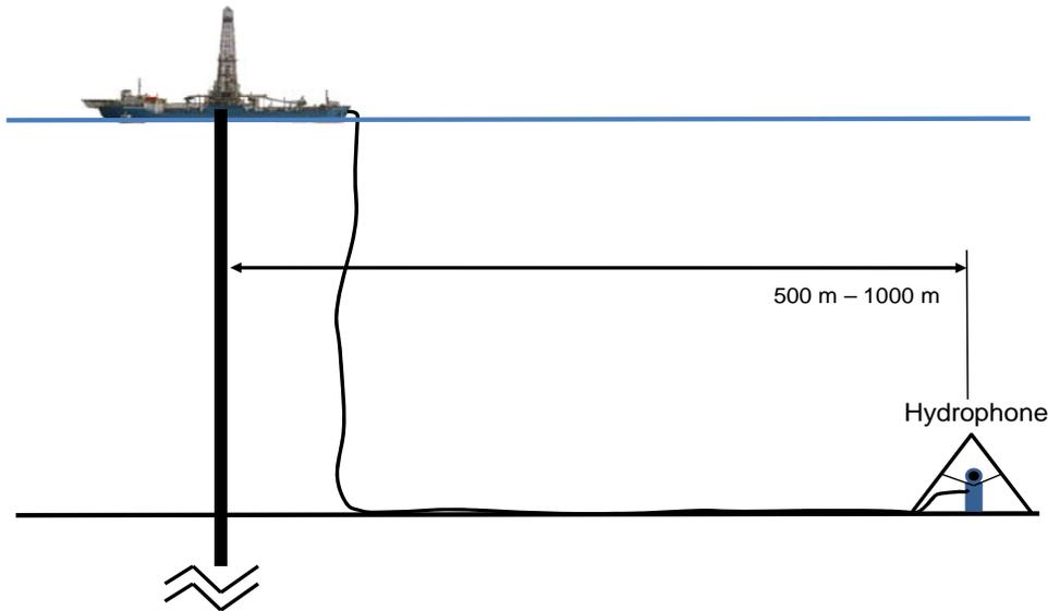
**Figure 1. Cabled hydrophone method for real time monitoring of drilling sound energy.**
