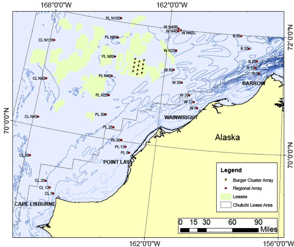
**Figure 7. Deployment locations of Hydrophones in acoustic arrays in the eastern Chukchi Sea, Alaska 2012. Depiction of hydrophone array at Burger is not scaled correctly based on description below (12 km by 18 km)**
